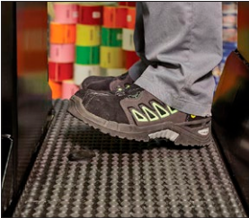
Foot switch for lowering the driver's platform
