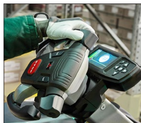
Multifunctional steering wheel with optional color display.
