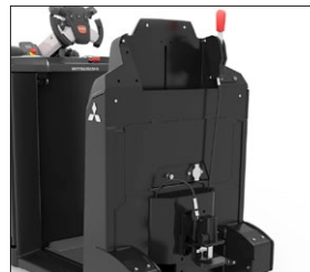
Automatic coupling with ergonomic unlocking handle
