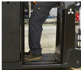
Suspended operator's platform.
