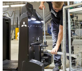
Manually operated trailer coupling
