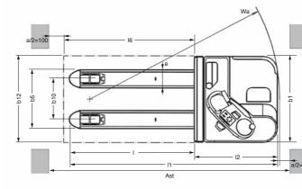
$\begin{array}{rcl} Ast &=& Wa + R + a \\ Ast &=& Working aisle width \\ Wa &=& Turning radius \\ a &=& Safety clearance = 2 x 100 \text{ mm} \\ R &=& \sqrt{(16 - x)^2 + (b12 / 2)^2} \end{array}$
